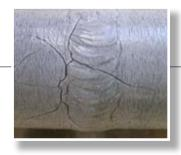
There are so many things one cannot see with the naked eye, but which we nevertheless need to have full control over. Where human safety is concerned, the smallest bolt needs to be intact and fulfil its function. With the Bycotest magnetic particles (MT), you can distinguish the harmless scratch from a dangerous crack.
